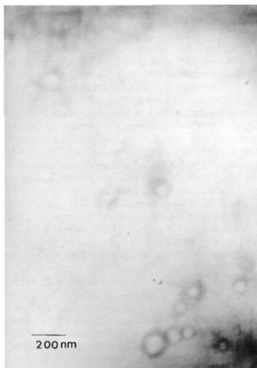
Figure 1. Transmission electron micrograph of vesicles of 1b , prepared via ethanol injection and examined as a frozen-hydrated sample ( -176^\circ\text{C} ; Philips 400 TEM instrument).
